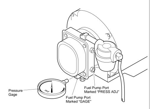
Figure 10 - Adjusting Pump Pressure
